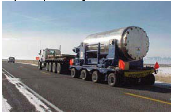
Figure 2. TMI core debris moved by truck and trailer from Test Area North (TAN) to INTEC.
